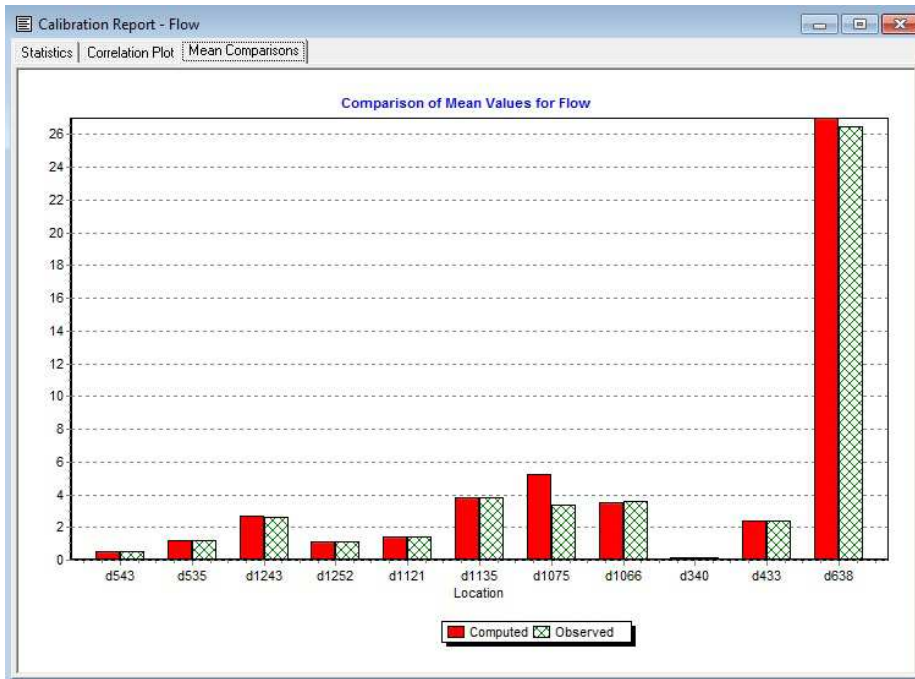
Fig. 7. Report on flow rate calibration – comparison of the mean observed flow values with the computed values at the individual measurement points
