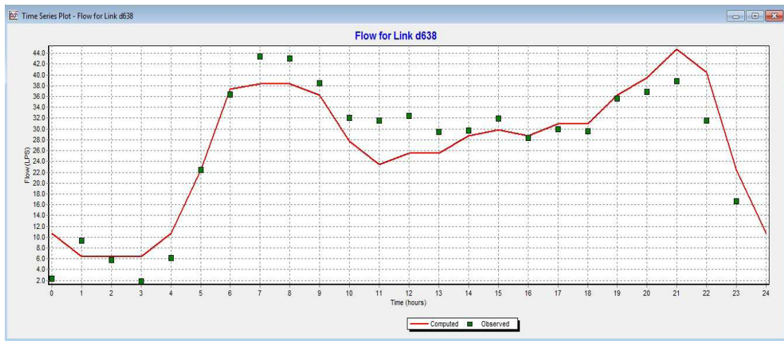
Fig. 10. The comparison of the process of changes in water flow rate, computed and observed, in pipeline d638
