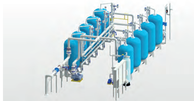
Pressure container de-ironing station in the Kostroma region 1400 m 3 /day
