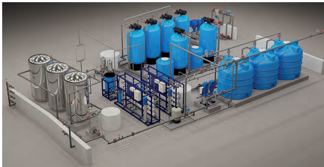
Automatic deep water treatment station, 6 m 3 /h or filling ice arenas, SOCHI 2014 Olympics
